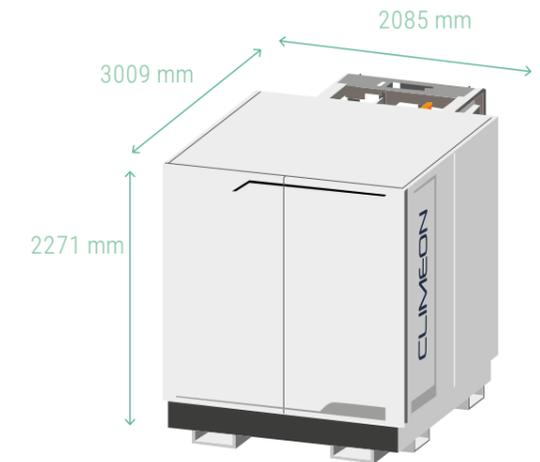
**Please note:** Space of 1500mm in front, 500mm above, and 691mm behind is needed around the module. 500mm is recommended between modules, when more than one module is present.
